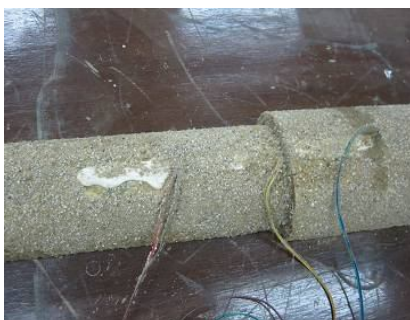
图 5 应变片布置 Fig.5 Arrangement of strain gages on piles
